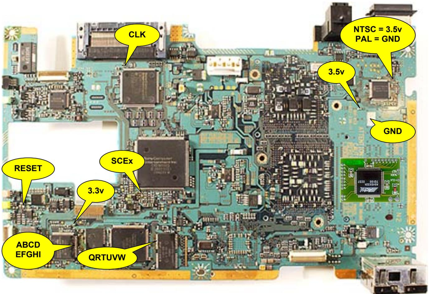
With reference to the above photo, solder wires to the **3.3v** and **GND** points. It is good practice to use thicker wire for power and ground and, of course, to insulate it.
