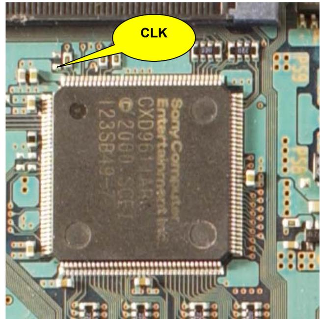
The **CLK** point is a pad above and to the left of pin 143 (see photo right). The **CLK** wire should be laid along the PS2 motherboard rather than allowed to run "in air". This is to ensure a proper ground plane to preserve the fidelity of the 36 MHz. Clock.
