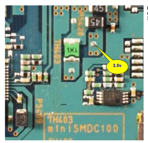
It is recommended that you use 23 swg = 22 awg wire for 3.vv / GND.
