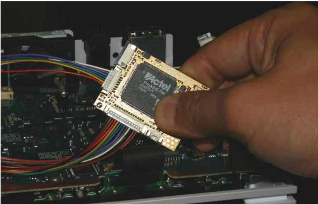
3) Connect the 2 wire eject cable connector to the eject signal assembly, and then to the eject 2 pin connector on the MOD.
