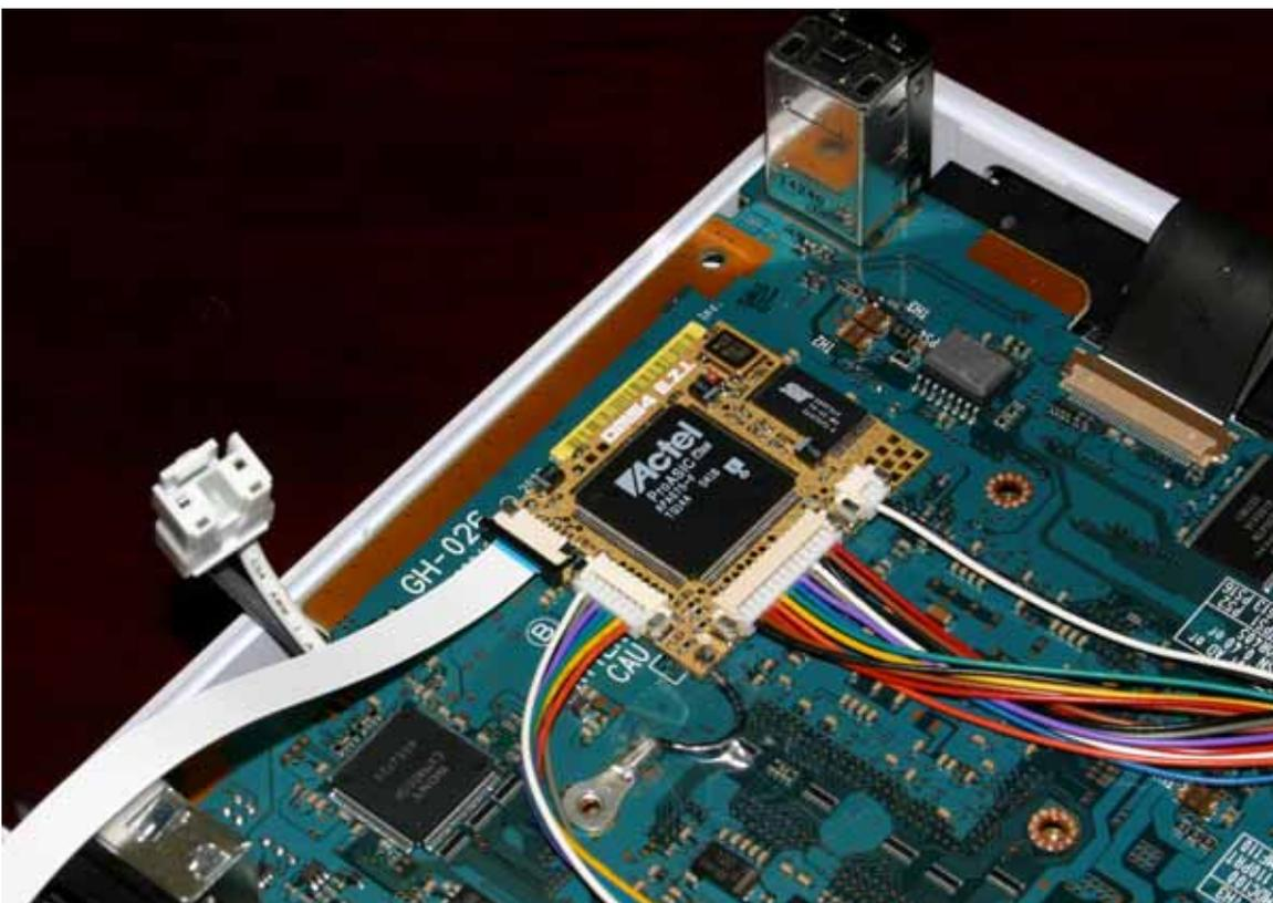
2) Connect the FFC cable to the E.Z.I. LED test panel.
