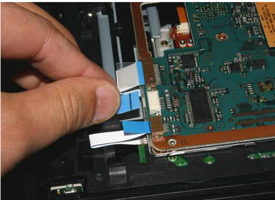
2) Connect the PS2 eject cable into the eject signal assembly.
