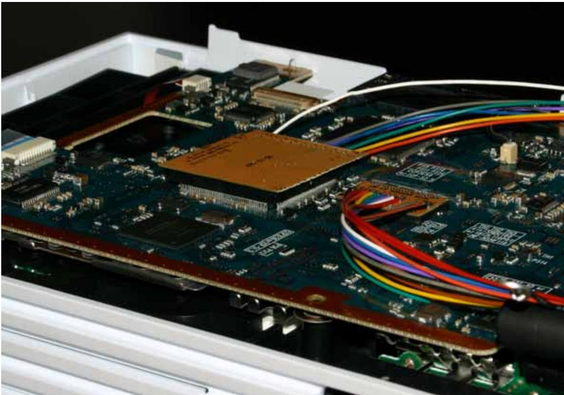
3) Make sure that the DSP clip has made a firm connection, by pressing down with both thumbs as shown in the photo.
