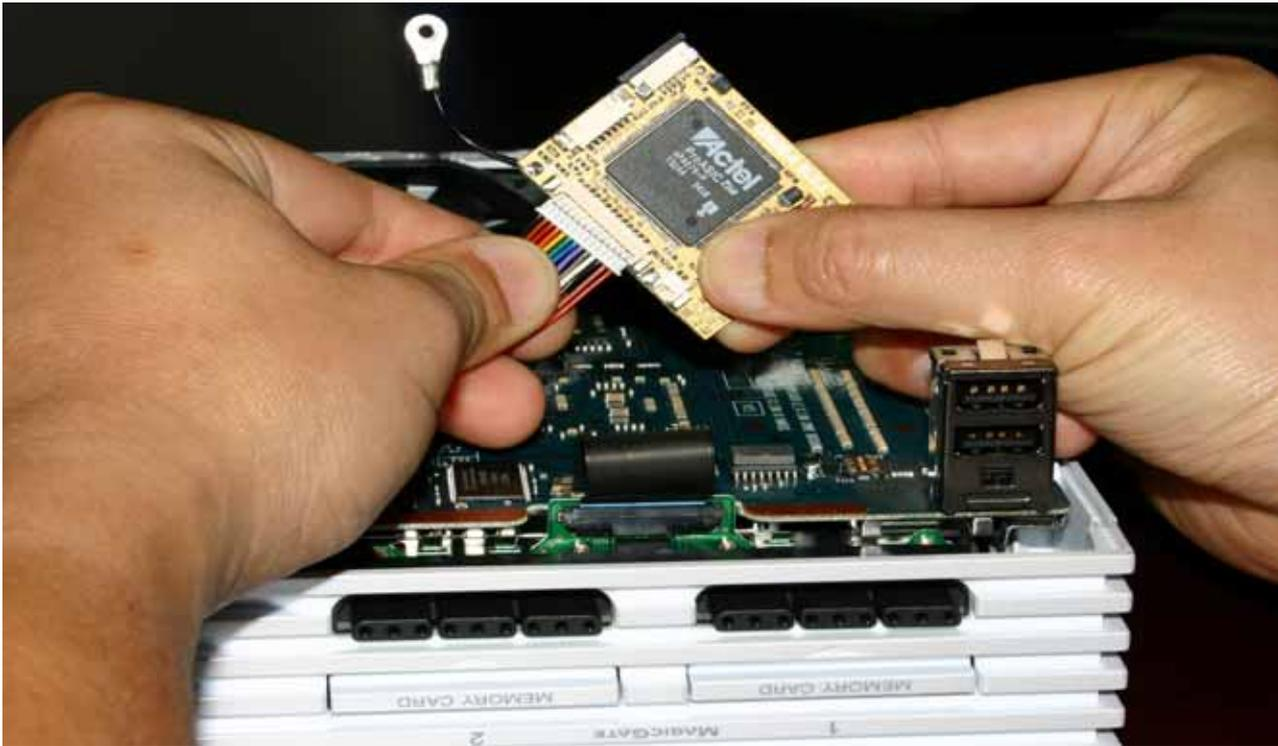
2) Connect the DSP cables next by mating the 7 wire DSP cable connector to the female 7 pin connector on the MOD.
