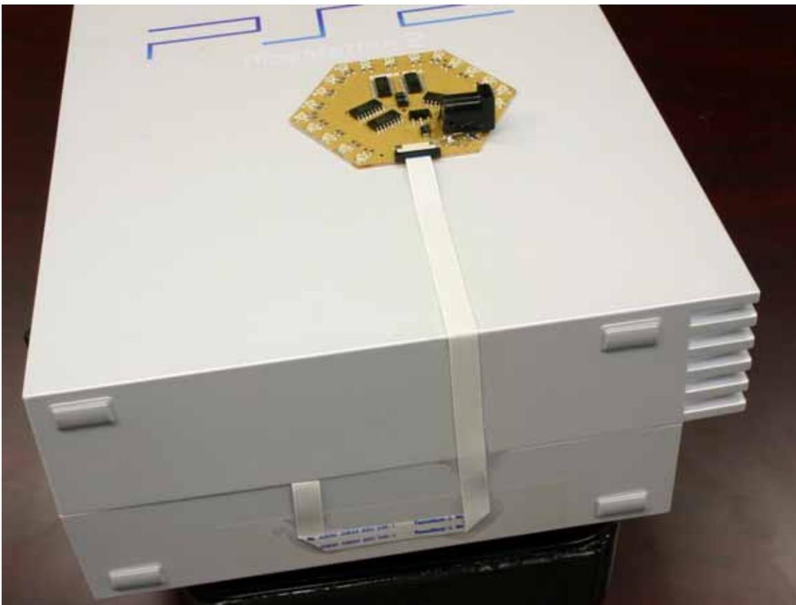
3) If you have connected the LED panel, connect a 9V DC (polarity: center = +ve) 2.5mm power jack P.S.U. (not included) to the jack on the E.Z.I. LED panel.
