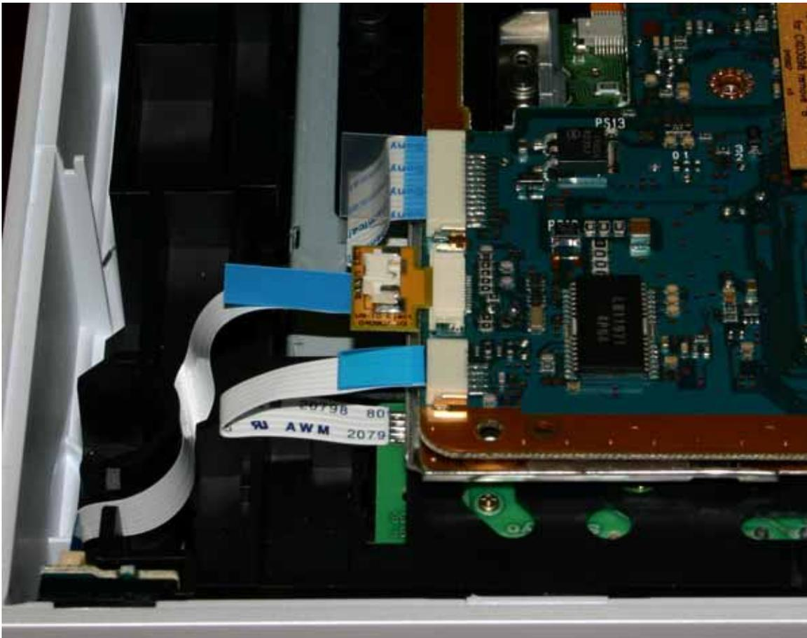
PLEASE TAKE GREAT CARE WHILST DISCONNECTING THE RIBBON CABLE NOT TO TEAR IT! PLEASE ALSO ENSURE THAT EXCESSIVE FORCE IS NOT USED WHILST CONNECTING THE EJECT ASSEMBLY TO THE CONSOLE.
