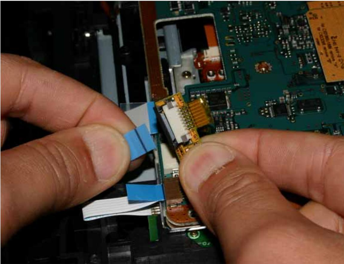
(Please note that the FFC connector on the underside of the V5-V8 PCB assembly is only to be used for V6 consoles!)
