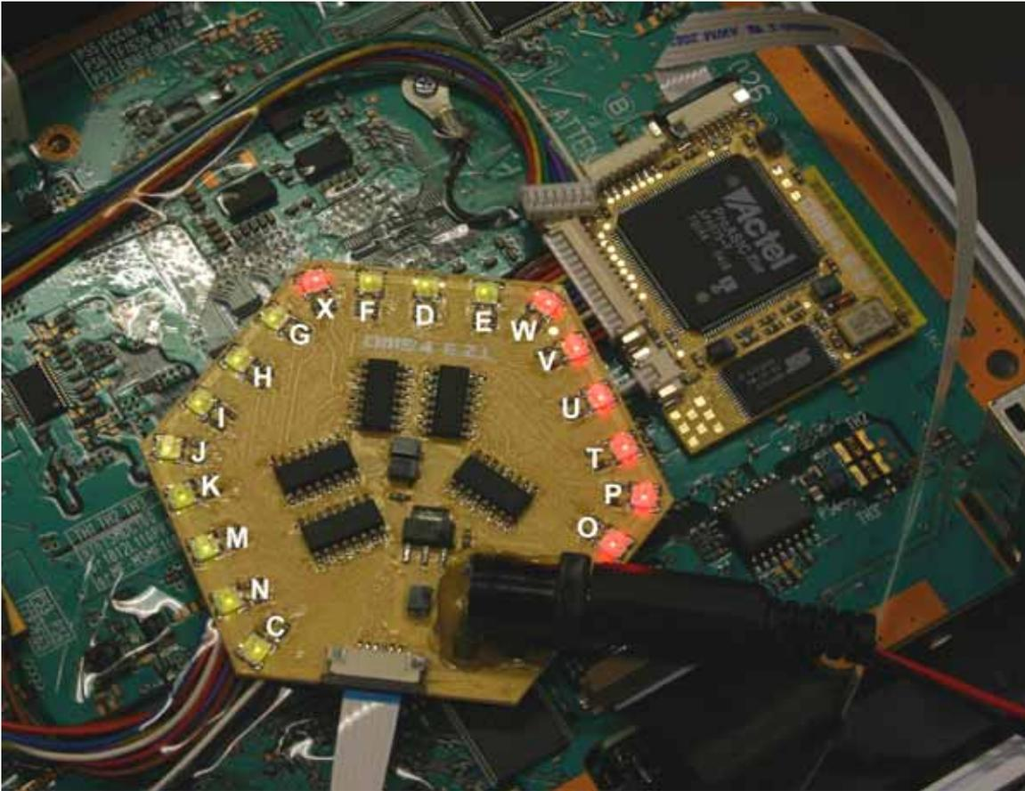
**NOTE:** Due to manufacturing error, the initial batch of LED panels shipped out did not have letters marked on the PCB next to each LED. In the case that you have one of these LED panels, the letter to LED mapping is shown above. The DMS4 EZI part which each led/letter corresponds to is as follows:
