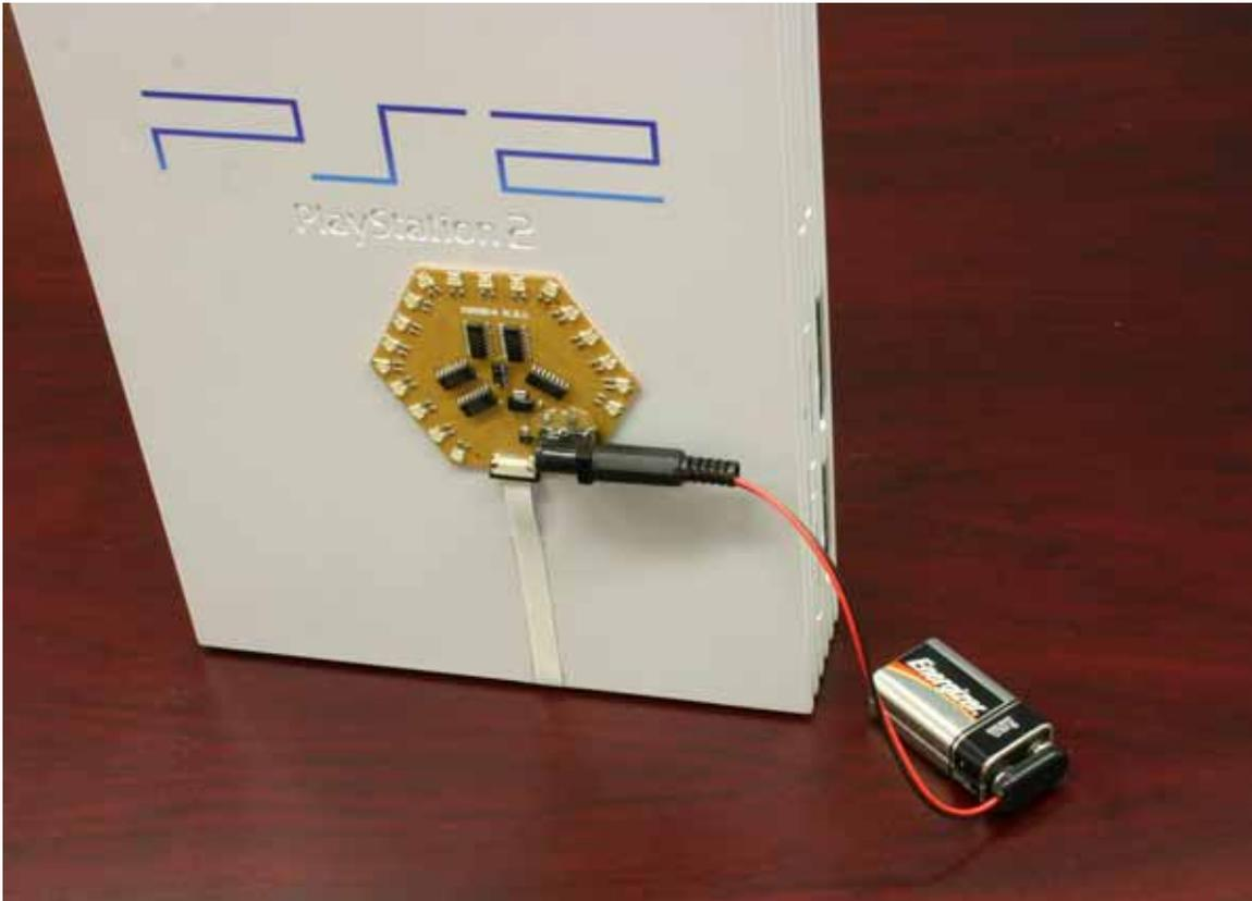
4) You can now test the functionality of the modchip. Installation is complete.
