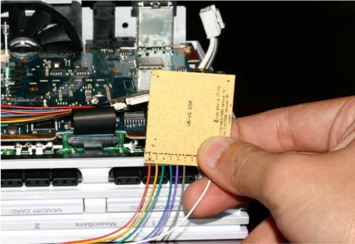
3) Align the DSP clip properly by situating the "PIN 1" marking on the DSP clip PCB over pin 1 of the DSP IC. Make sure that the edge of the clip is parallel to the DSP on four sides before connection. Please ensure that the DSP clip is situated equally over each side, as this is paramount to proper connection.
