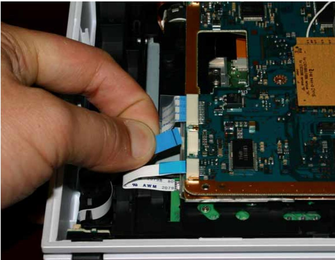
2) Connect the PS2 eject cable into the eject signal assembly.
