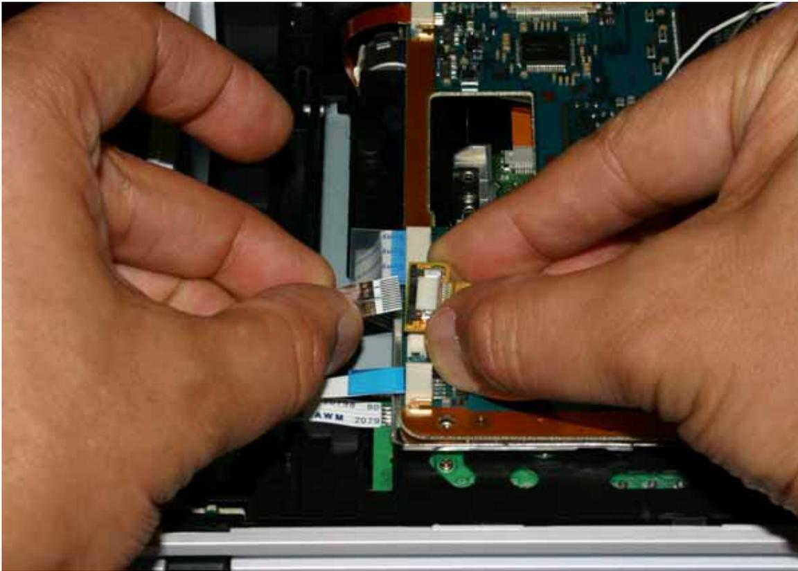
3) Connect the eject cable assembly to the connector from which you removed the ribbon cable.
