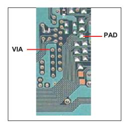
With reference to the picture on the left, it is straightforward to solder a wire to a **PAD**.
