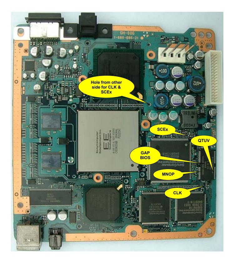
It is recommended that you solder to the PS2 motherboard first and then connect each wire to the appropriate point on the Messiah 2.
