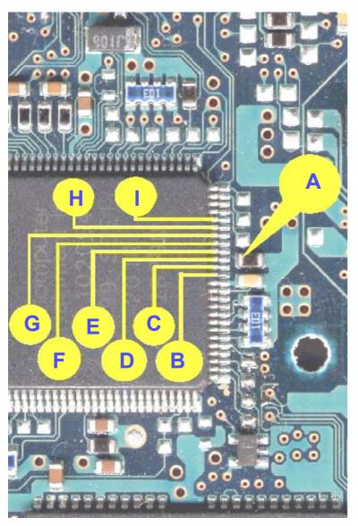
With the "easy" points now connected on the PS2 motherboard, you will need to solder the wires to CD/DVD Controller (points **ABCDEFGJHI**) and later, the BIOS chip (points **MNOP QTUV**).
