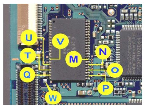
Note that there are **9** wires associated with the Non-GAP BIOS, with **W** co-located with the other wires.
