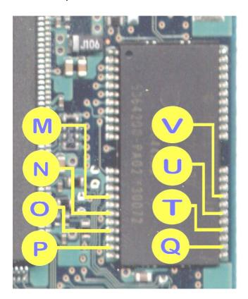
When the soldering is complete, take the wires through to the top side of the PS2 motherboard. You may care to place a sticky identification label onto each wire to ensure that it is correctly connected to the Messiah/Clone. Alternatively, connect each wire in turn to the Messiah/Clone; this will ensure you don't cross-connect any wires.
