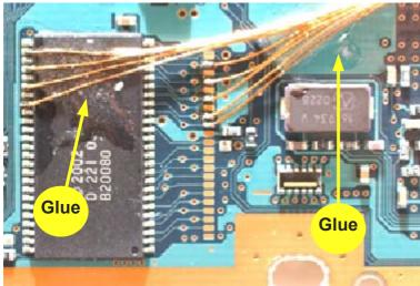
You may care to place a sticky identification label onto each wire to ensure that it is subsequently correctly connected to the Messiah 2. Alternatively, connect each wire in turn to the Messiah 2; this will ensure you don't cross-connect any wires.
