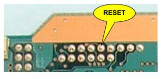
Install these points first. Note that **3.3v** & **GND** are 23 swg = 22 awg insulated stranded cable. The **GND** pad is covered with lacquer that must be scraped off or the lacquer removed with flux spray as described in the <u>soldering</u> section.
